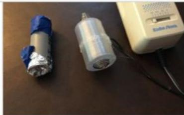
**Battery Eliminator from a recycled wall wart**
