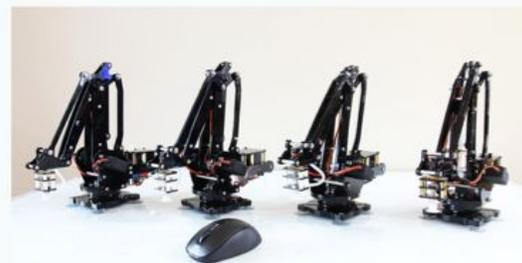
uArm is an Arduino-powered desktop 4-axis parallel-mechanism robot arm, modeled after the ABB industrial PalletPack robot.
