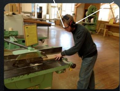
Ensure there is no loose clothing or hair that can get caught in the machine Safety shoes must be used to prevent injury from any objects dropping from the bench.
